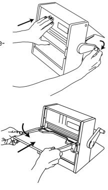
Remove used supply cartridge by pulling outward. If there is film between the rollers. turn handle counter-clockwise.
